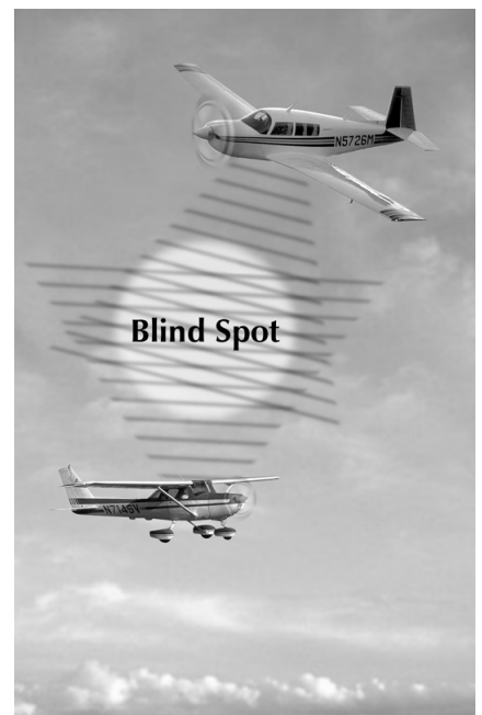
This picture illustrates where the blind spot is below a Piper and above a Cessna. Please be aware of your surroundings while in the air. Recognize what is above and below you at all times.
